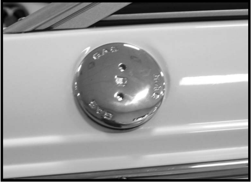
Fuel Fill Fitting
