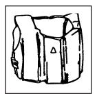
• **TYPE III-** Known as a flotation aid it is good for calm, inland water or where there is a chance for quick rescue. It is designed so wearers can place themselves in a face-up position in the water. The wearer may have to tilt their head back to avoid turning facedown in the water.
