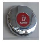
The fuel fill is labeled "gas" and is located along the starboard aft deck. When fueling it is important to keep the fill nozzle in contact with the fuel fill line since it decreases static electricity, which may spark and ignite gasoline vapors. Always use the recommended fuel octane rating as specified in your outboard engine owner's manual. Extinguish all flame
