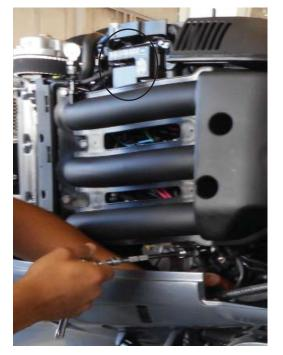
As part of Yamaha outboards under the motor shroud (engine cover) on the port side of the outboard engine is an electrical cover. Inside this cover is a variety of fuses protecting various engine components. There are also extra fuses stored along with a fuse puller. For further information, refer to the manufacturer's outboard engine manual.
