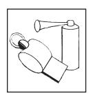
According to both Inland and International Rules, all boats **must** carry some way of producing an efficient sound signal. If your vessel is 12 meters (39' 4") or longer, a power whistle, power horn or bell must be carried. The bell must be 7 7/8" in diameter.
