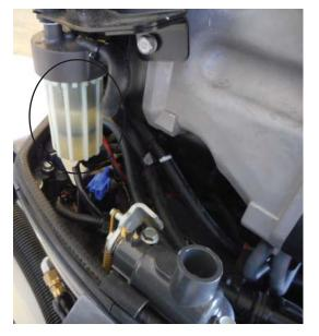
As part of Yamaha outboards under the motor shroud (engine cover) on the lower port side of the outboard engine is a fuel filter. Periodically check to ensure the fuel filter is clean and free of water. When reinstalling the filter tighten to manufacturer's specifications. Check for leaks after starting the engine. For more information refer to the
