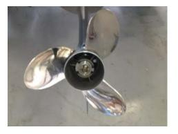
Out-of-balance or nicked props will effect performance or cause vibration. Damaged props should be replaced, but those that are chipped or bent can usually be reconditioned by a marine dealer or a propeller repair facility. When cruising, consider carrying a spare set of props on board
