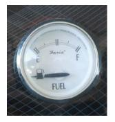
The fuel gauge indicates the level of fuel inside the fuel tank sent by the fuel sender. It is a good idea to keep the fuel tank "topped off" when possible to reduce fuel vapors inside the tank. Do not run your fuel too low as this style gauge is not always accurate. Always allow for a "safety" factor. Remember that the Garmin is not set up to monitor fuel tank levels. The dash gauge
