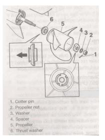
Removing the propeller- Before removing the propeller make sure the remote control is in neutral and the ignition keys are removed to prevent the outboard engine starting and possibly causing bodily injury. Always wear gloves when removing or installing propellers since the component blades are very sharlp.
