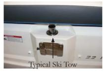
A water sports ski tow is located center line at the stern deck. Double loop the line first through the hole and then around the ski pylon and cinch it tightly. This procedure helps to keep the line intact when there is no strain on it.
