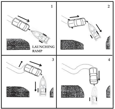
A trailer backs in a direction opposite to an automobile. In 1, driver swings the rig near the launching ramp. In 2, the driver cuts the vehicle toward the driveway. In 3, the driver cuts the vehicle wheels to the left and then backs into the ramp as the trailer moves to the right. In 4, the driver straightens the vehicle wheels to follow the trailer as it backs down the ramp.
