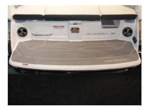
As an option SeaDeck® is featured on select vessel swim platform and walk through areas. The non-skid, closed cell material is derived from UV protected non-absorbent foam. You will find the product easy to clean with a high stain resistance.
