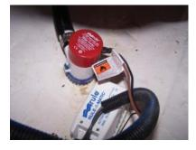
The bilge pump is usually installed in the bilge. Normally the unit features an automatic float switch. Periodically check for foreign materials stuck in the strainer area or discharge hose.
