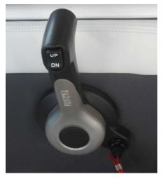
Check the helm control box and the cable attachment at the engine for tightness and shifting without binding. Shift and throttle controls at both the engine and helm areas must be checked on a periodic basis. At the engine end, make sure all control cable hardware is tight and control cable brackets are secure. An application of silicone spray on the cable ends periodically will keep control
