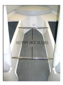
To use the bow filler cushion locate the support bars found under the bow cushions. One is longer than the other. Make sure both bars are seated in the liner detents (Typical bow seating shown).
