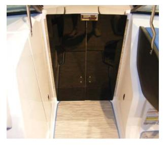
Optional walkthrough bow doors are great in foul weather. With the tonneau (bow) cover in place, simply open the doors and pull across the bow opening. Secure shut. Close the tonneau cover.
