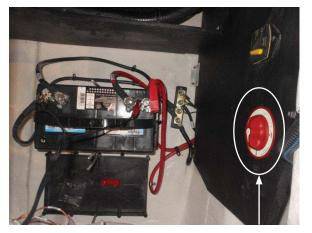
As an option your vessel may utilize a dual battery switch which controls 2 batteries located in the port aft outboard engine storage locker. This can be accessed by removing the port aft transom cushion. With this style switch, the
