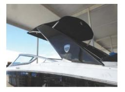
As an option the Power Tower hinges forward for tight overhead clearances such as bridges and restricted storage situations.
