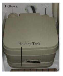
chemicals, paper is available, and the holding tank is empty. To fill the toilet follow the manufacturer's recommendations for mixing the solution. Use the fill to pour in the deodorant chemical and water. By pushing down on the bellows the chemical mix in released to rinse and help flush the toilet bowl. When the flush valve is pulled forward the toilet bowl waste water empties into the holding tank. Close the flush valve after each use.
