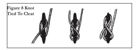
A useful knot to learn for general docking is the figure eight with one end reversed. By turning the free end of the line back under, the knot can be released without disturbing the boat. After some practice one person can secure a vessel easily to a dock or pier in a variety of weather conditions. This knot normally is used to tie the bow and stern. Then the vessel can further be fastened by tying the spring line in the figure eight knot. Wrap it around the cleat 2 or 3 times. 5-26
