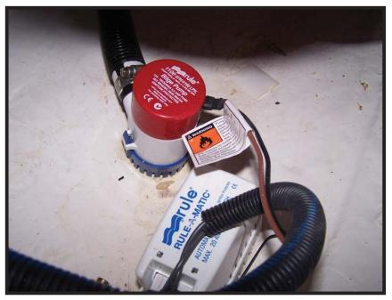
Typical Bilge Pump And Automatic Float Switch
