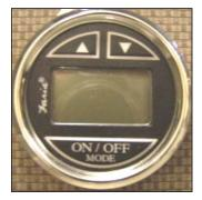
The depth gauge indicates the water depth under the keel of the boat. It features a shallow water alarm to warn the skipper of hazardous situations. By monitoring the water depth, damage to props, and underwater hardware can be avoided. This gauge is connected to a transducer on the bottom of the hull, accessible through a removable plate in
