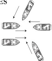
In a head-on meeting, both vessels must sound a single blast to give way toward starboard and pass to port.
