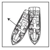
Outboard boats have the ability to angle in or out their drive unit in relationship to the transom. This is accomplished by hydraulic shocks located on the lower unit housing along with an electrical sender unit that reads the drive angle and sends information to the dash trim gauge showing a reading.
