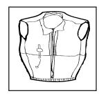
• **TYPE V-** This is the least bulky of all PFD's. It contains a small amount of inherent buoyancy, and an inflatable chamber. It is rated even to a Type I, II, or III PFD (as noted on the jacket label) when inflated. Hybrid PFD's must be worn to be acceptable. equipment.
