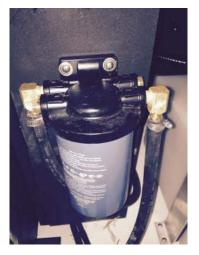
Fuel filters are installed on outboard engines. Normally there is a fuel filter under the motor shroud (cover) which should be serviced per outboard motor manufacturer. Also, Regal installs an in-line 10 micron water separator filter which is a spin on type similar to an automobile oil filter. Its main purpose is to trap dirt particles and condensation in fuel. It is a good idea to keep an extra fuel filter on board along with a filter wrench, catch container and clean rags for
