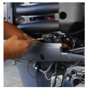
Your Yamaha outboard features a flushing device which when connected to a garden hose circulates fresh water through the engine to purge unwanted debris such as found in salty, brackish, and silty water.
